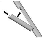
4. Now push the top part of the battery into the frame, until you hear the battery lock into position, and push the limiting stopper to keep the battery from dropping.
