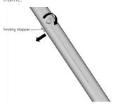
Then push the limiting stopper up to release the second locking mechanism and hold the two sides of battery to pull the battery.
