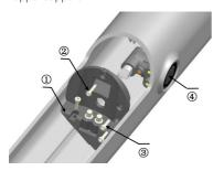
Hold the two sides of battery and place the bottom part of the battery into the frame, making sure it sits comfortably on the down support.
